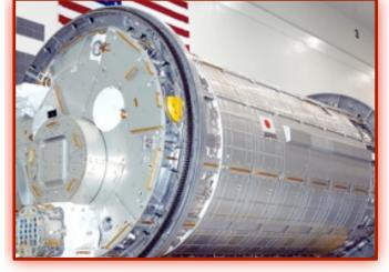
The second part of the Japanese module Kibo is preparing to be fitted into the Space Shuttle for launch to the ISS.
