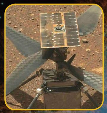
NASA's Mars helicopter Ingenuity has begun to scout missions for the Perseverance rover, completing its ninth and most challenging flight yet. Flight nine included a speed record for the aircraft at roughly 11 mph, which NASA called "a high-speed flight across unfriendly terrain, which will take us far away from the rover."
